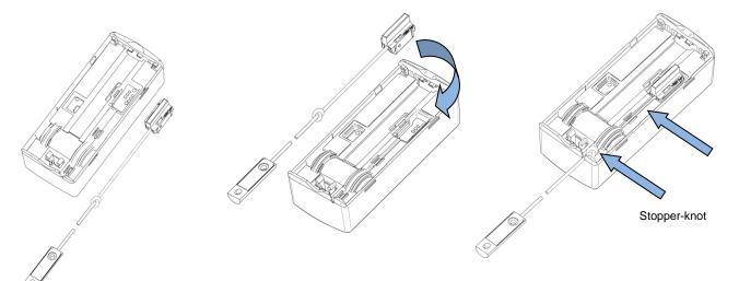
Return the heat cost allocator and plug the connector of the remote sensor into the interface inside the heat cost allocator.
