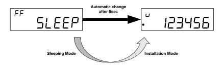
The  $\bullet$  symbol indicates that the heat cost allocator is in installation mode.
