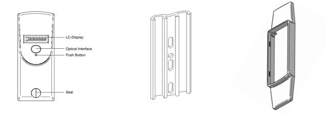
Standard aluminium back plate for nearly all existing bolts with common dimensions and mounting possibilities – thus easy installation
